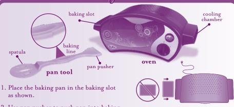
2. Use pan pusher to push pan into baking chamber. Stop when the baking line on the handle lines up with the bottom edge of baking slot as shown. Do not use your hands to push pan in. Do not leave pan tool in oven.
